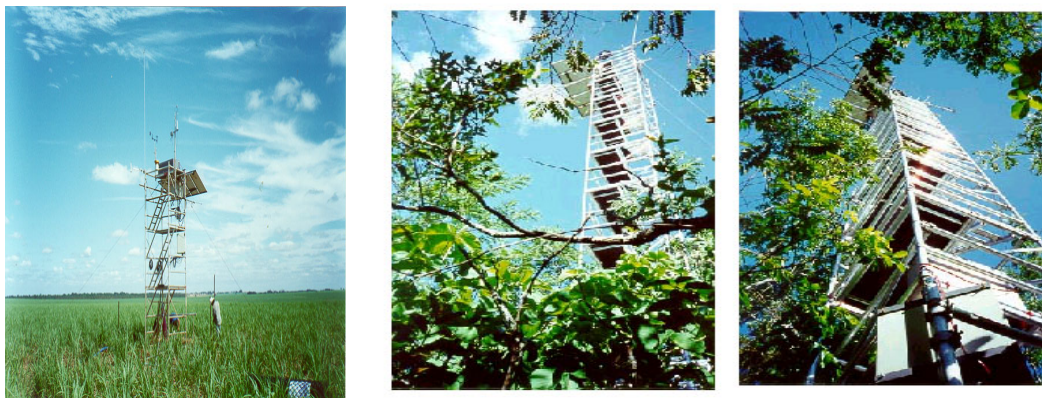
Figure 1: Implemented tower with eddy correlation and meteorological instrumentation at sugar cane (left) and Cerrado (center, right) sites.
